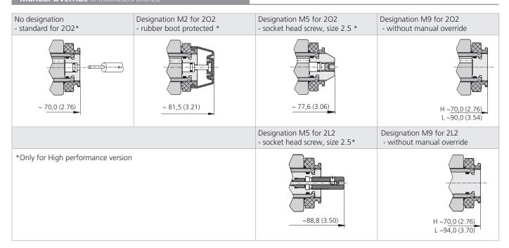
In case of solenoid malfunction or power failure, the spool of the valve can be shifted by manual override as long as the pressure in port T does not exceed 25 bar (363 PSI). For alternative manual overrides contact our technical support.
