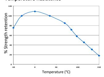
"Hot strength" shear strength tests performed on mild steel. 24hr cure at
