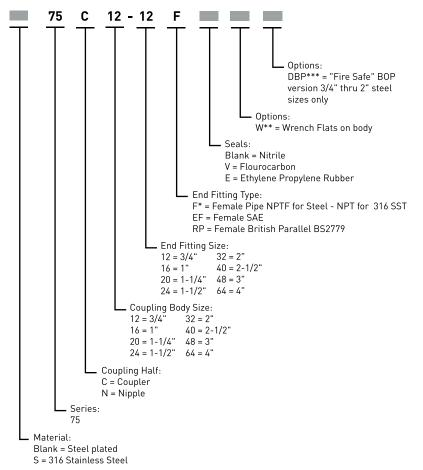
\* For sizes up to 3", NPTF threads. For sizes over 3", NPT threads.
